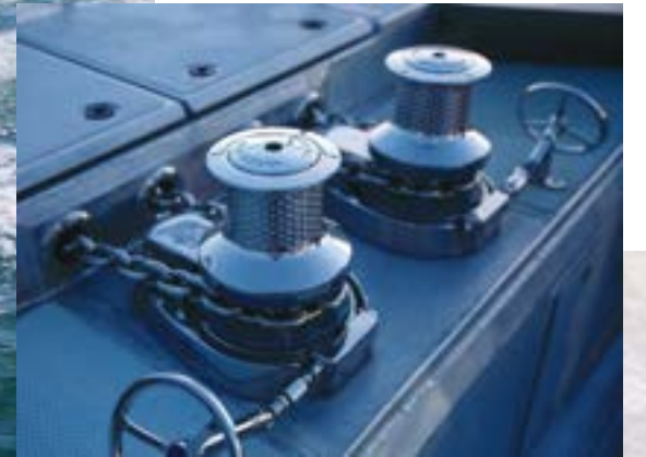
The unfinished aluminium exterior will patina nicely over time. Much like a commercial vessel, the Arksen 85 boasts heavy-duty winches and wide side decks with hidden storage in the bulwarks
