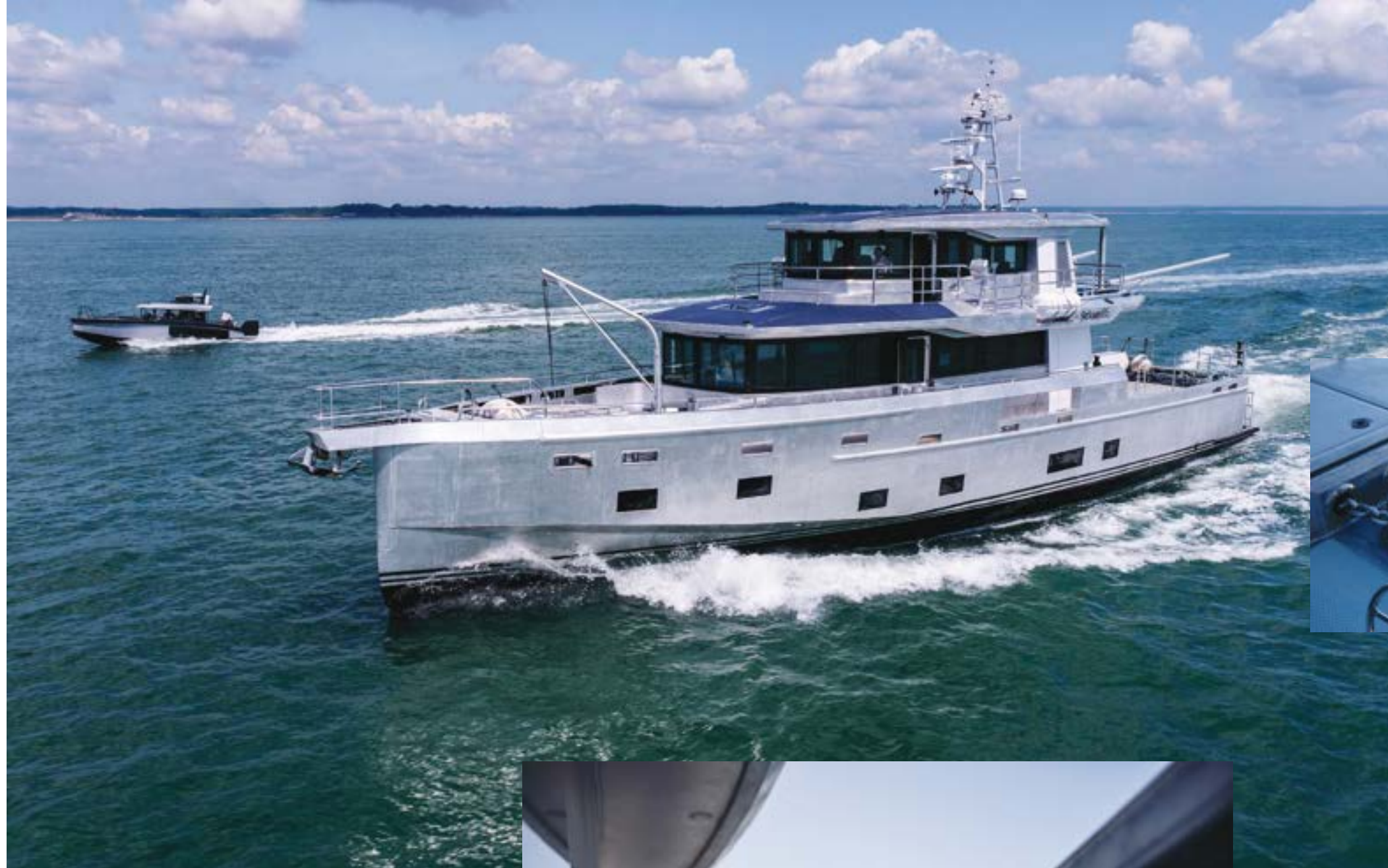
The unfinished aluminium exterior will patina nicely over time. Much like a commercial vessel, the Arksen 85 boasts heavy-duty winches and wide side decks with hidden storage in the bulwarks
